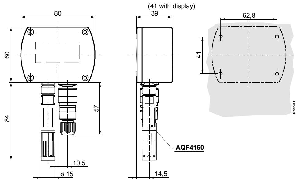
Dimensioning without (with) LCD-display
